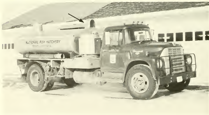
FIGURE 111. Aluminum elliptical tank with refrigeration unit mounted at the front. Aeration is by gas-driven pumps and pure oxygen. Note air scoops (arrow) for CO 2 removal on front and rear of tanks. (Ennis National Fish Hatchery, FWS.)
