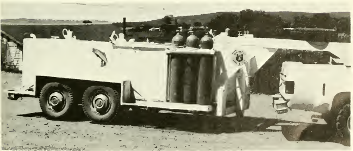
FIGURE 108. Fish distribution tank mounted on a gooseneck trailer. This unit can be pulled by a pickup truck.
