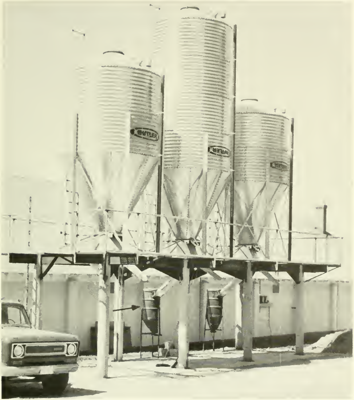
FIGURE 74. Bulk storage of pelleted fish feeds. Dust and "fines" are screened out and collected (arrow), and can be repelleted. This type of storage is preferred to bins that require augering the feed up into a truck, because augering breaks up the pellets. (FWS photo.)
