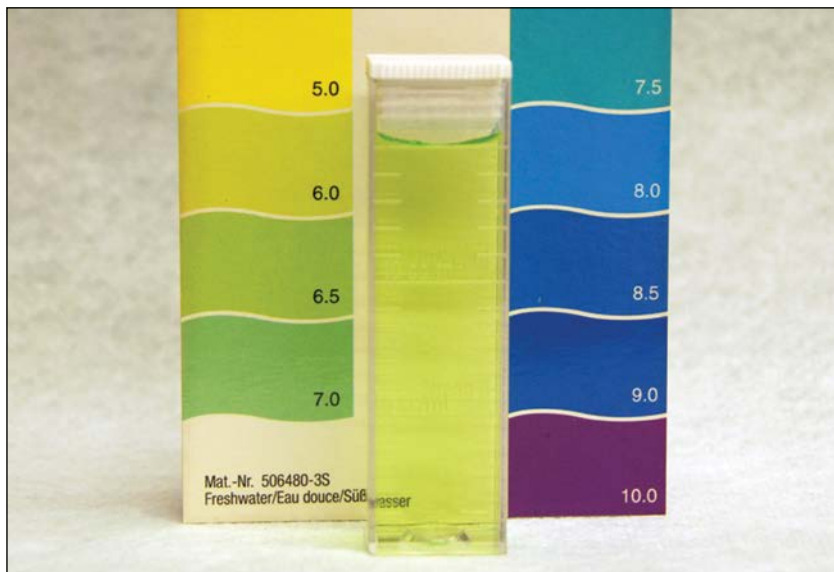
Figure 2.1 Water sample tube (center) with pH color comparator chart. (TetraTest, Spectrum Brands, Blacksburg, VA.)
