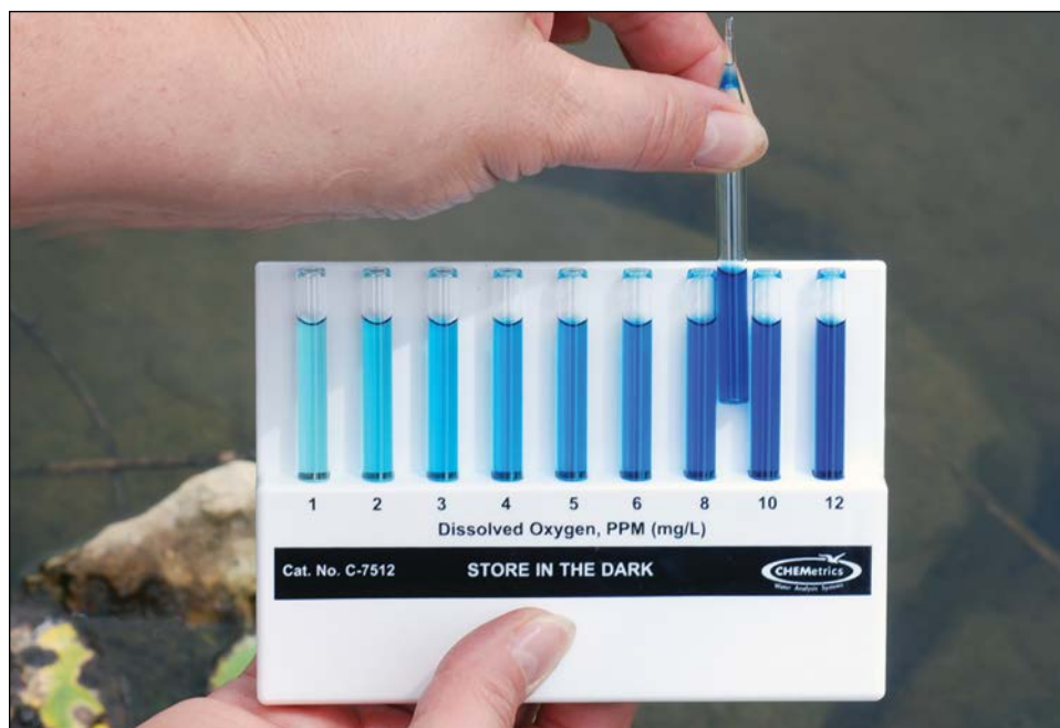
Figure 2.8 Sample ampule with color comparator for analyzing dissolved oxygen concentration. (CHEMetrics Inc., Midland, VA.)
