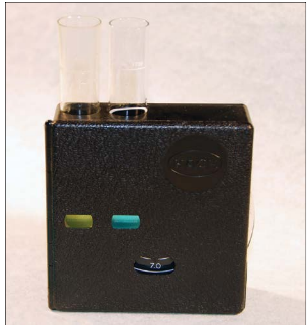
Figure 2.5 Standard blank (right tube) and test sample (left tube) color comparison method with pH color disk. (HACH Company, Loveland, CO.)
