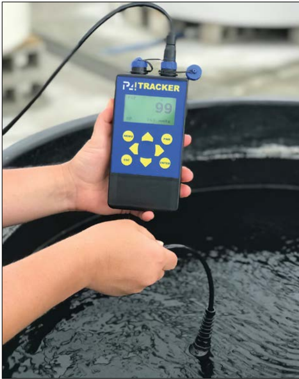
Figure 2.12 Saturometer and probe. (Point Four Systems, Inc. Pentair Aquatic Eco-Systems, Apopka, FL.)
