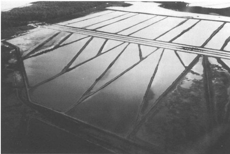
Figure 3. Aerial view of semi-intensive farm in Ecuador. A triple reservoir canal delivers water from the pump station (upper left) to nursery and growout ponds. Three-phase nursery/growout ponds are shown below the reservoir canals.
