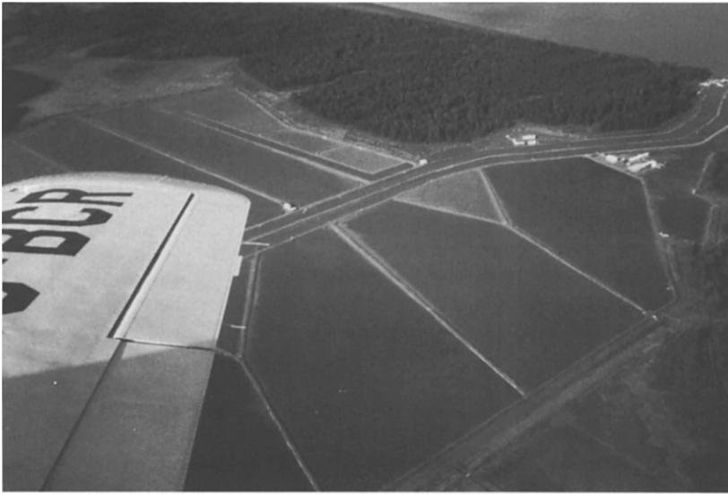
Figure 2. Aerial view of semi-intensive farm in Ecuador. A reservoir/canal delivers water from the pump station (upper right) to nursery and growout ponds. A drainage ditch at the opposite end of each pond returns effluent water to the source.
