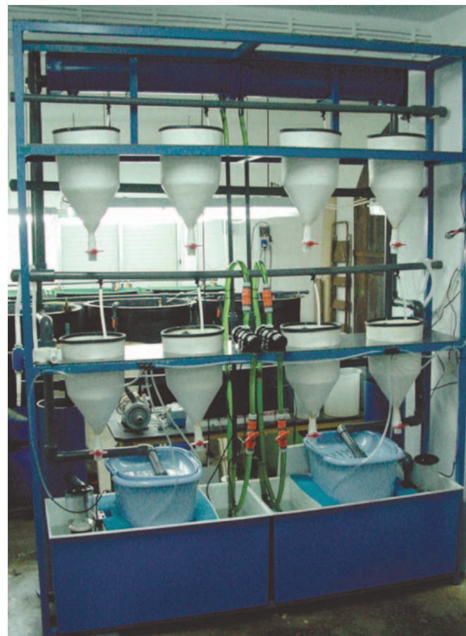
Color Plate 7 Larval culture system for marine ornamental decapods at Laboratório Marítimo da Guia, Faculdade de Ciências da Universidade de Lisboa using small-scale research tanks (10 liters) (photograph by the author).
