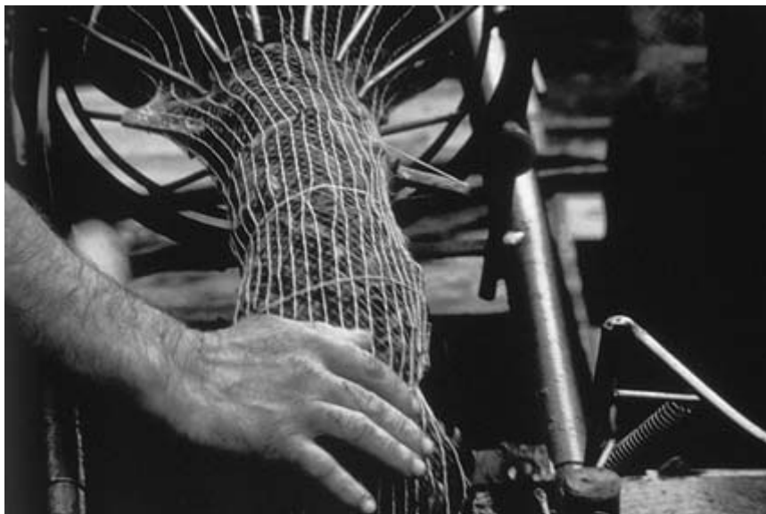
Fig. 7.9 Sleeve for feeding mussel spat into mesh stockings. (Photo: Sea Fish Industry Authority).
