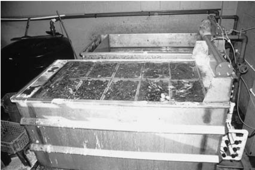
Fig. 12.5 750kg multi-layer mussel purification tank. (Photo: D. B. Edwards).
